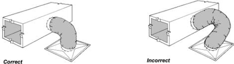
2. Avoid bending ducts across sharp corners or incidental contact with metal fixtures, pipes or conduits. Radius at center line shall not be less than one duct diameter.
